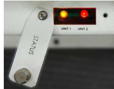
Figure A-2. Faulted System Example
